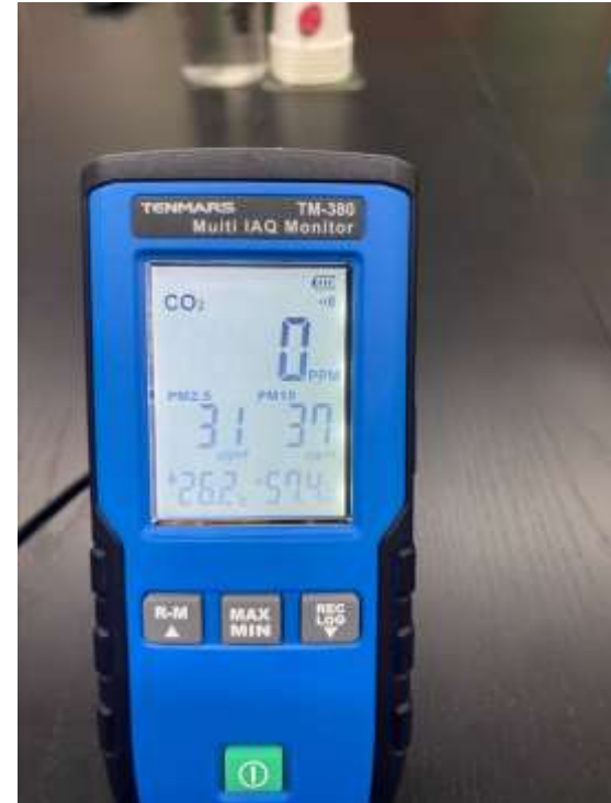
Indoor Air Quality monitor
